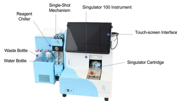
**Figure 1.** Singulator™ 100 System, including the Singulator instrument, single-use cartridge, chiller for nuclei reagents, and Single-Shot Mechanism for cell preparation reagents.
