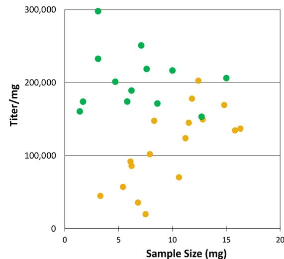
**Figure 5.** Dissociation of small samples with the NIC+ cartridges. Yield of mouse kidney nuclei per mg vs. sample size is shown for standard (yellow) and NIC+ (green) cartridges.
