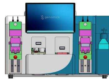
**Figure 2.** Singulator™ 200 System for processing two samples in single-use cartridges, with integrated chiller for nuclei reagents, and dual Single-Shot Mechanisms for delivering cell preparation reagents.
