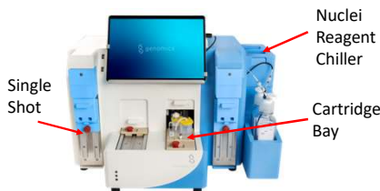
Figure 2. Singulator™ 200 System for processing two samples in single-use cartridges, with integrated chiller for nuclei reagents, and dual Single-Shot Mechanisms for delivering cell preparation and other reagents.
