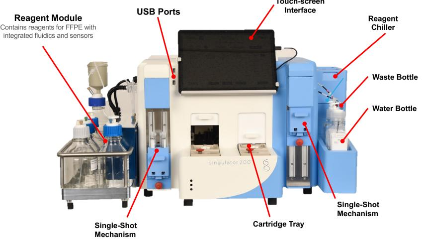
Singulator 200+ System, including Figure 1. Singulator the instrument, single-use cartridge, chiller for nuclei reagents, Single-Shot Mechanism for cell preparation reagents, and Reagent Module for FFPE reagents.
